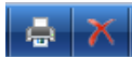
In the better example, the Delete command is physically separated from Print.
